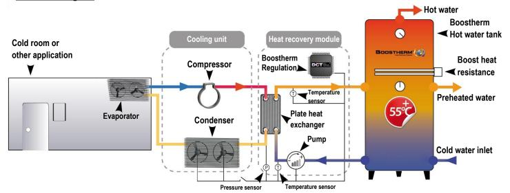
Boostherm operates according to 2 successive functioning modes during the same refrigeration cycle.
