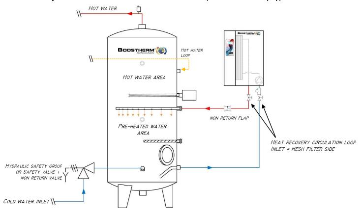
Assembly with a buffer tank in series with the installation water heater (or another DHW production station).
